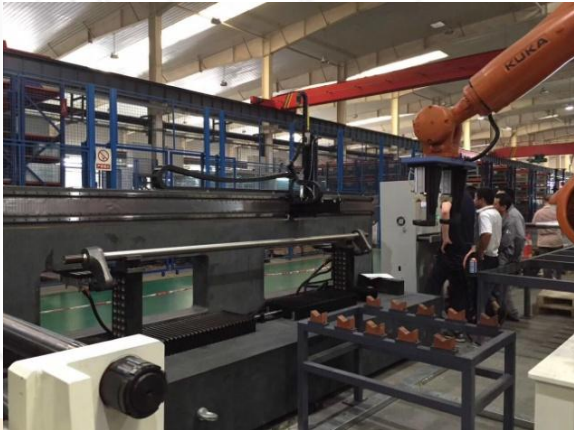
China Railway High-speed (CRH) Torque Rod Testing Equipment 4000*2000*450
